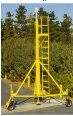
Model 745B Tail Support Stanchion Flyaway, ULD Type Unit
