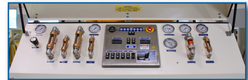
Malabar Coolant Service Cart control panel
