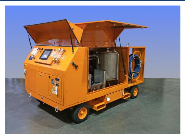
The Malabar Model 1016 A350 SCS Fill/Drain Cart is designed in accordance with Airbus system and equipment engineering specifications to meet the special servicing requirements of the aircraft supplemental cooling system. The unit has the controls and capacity to perform aircraft system coolant drain, fill, clean and de-aerate operations.
