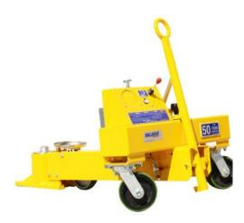
The Model 50P9AR Auto-Retract Axle Jack is a 50 ton capacity, two stage hydraulic jack designed primarily for use in jacking the main and/or nose landing gear of various aircraft. The jack consists of a two stage cylinder assembly, frame/reservoir assembly, valve block assembly, hand pump assembly and control console.
