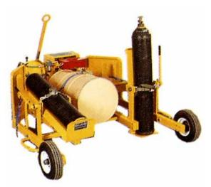
The Model 8776A Fluid Dispensing Trailer for Turbine Oil/Petroleum Based Fluids is designed to service all narrow and wide body aircraft. This modular and low profile fluid service unit reduces aircraft fluid servicing time. The unit dispenses fluid directly from the original 55 gallon drum, thus eliminating fluid contamination. The versatile system is suitable for synthetic turbine oils and petroleum based hydraulic fluids.
