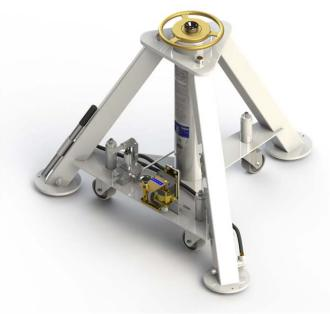
The Model 8964 Tripod Jack is a 20 ton capacity single stage hydraulic jack designed for use in aircraft maintenance. It consists of a tripod structure with integrated dual-leg reservoirs, hydraulic cylinder assembly, hand pump, swivel casters, locknut with handwheel and optional air pump with remote air inlet for remote air manifold operational control and a deadman air valve for individual jack operation.
