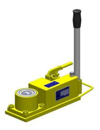
The Model 642S Axle Jack is a 12 ton capacity, two stage hydraulic jack designed primarily for use in jacking main and/or nose landing gear of various aircraft. The jack consists of a three stage cylinder assembly, hydraulic reservoir and hand pump assembly. Lifting handle is also supplied for ease of handling.
